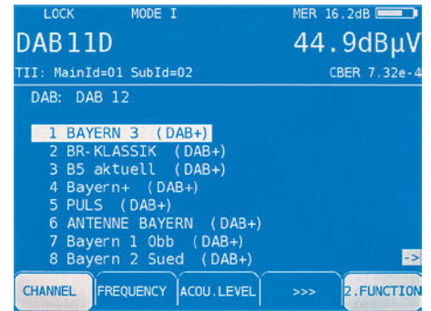
Measurement of the DAB + transponder 11D with level, MER and channel BER.
