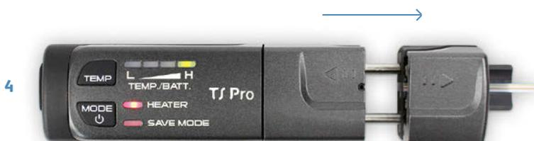
Pull the fiber holder part out of the main body and open it to check the stripped fiber.
