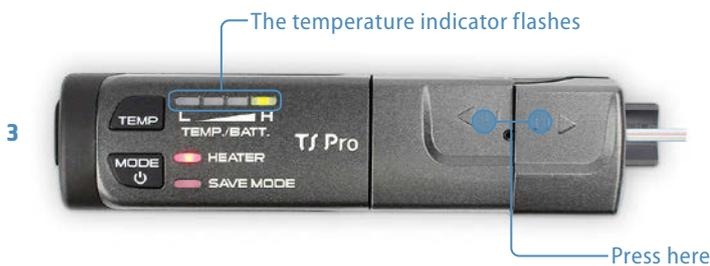
Press the covers and wait for temperature indicator to flash and the TS-Pro to beep.
