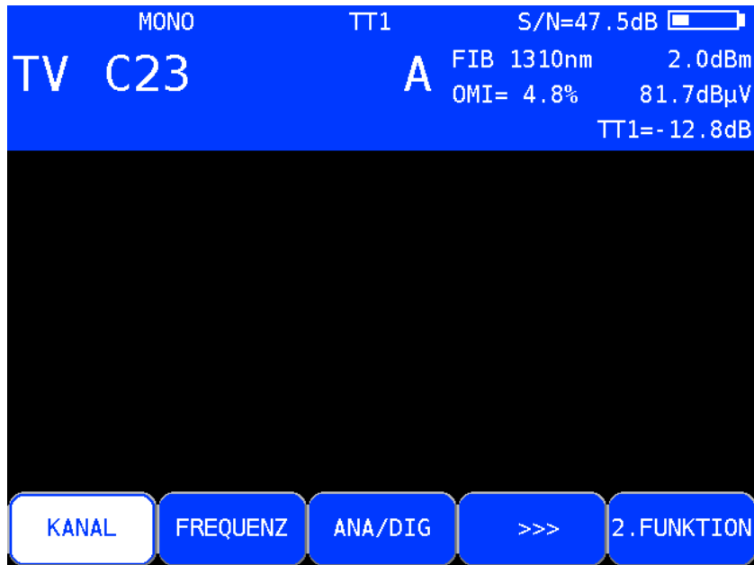
Optical power measurement
