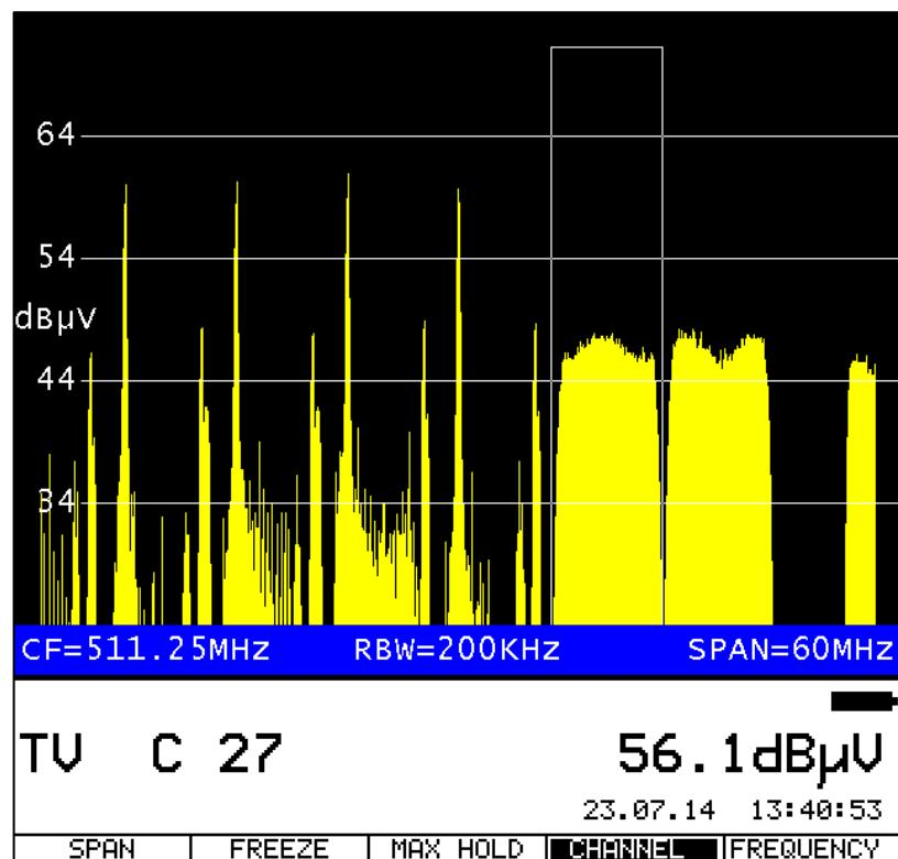
The comparison with the measured value displays in both cases with tuned measuring receiver shows that with activated Channel Mode in the analyser the levels are accurately reproduced.
