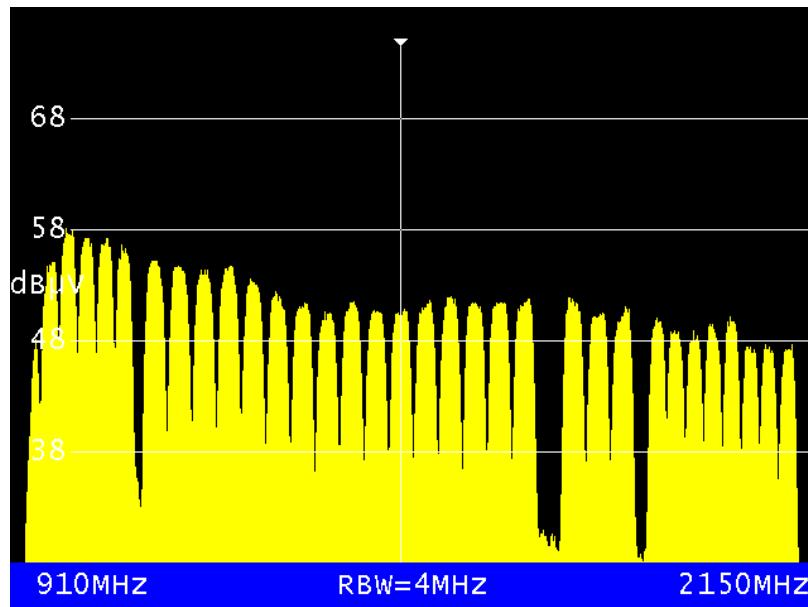
The SPAN here is 1240 MHz (2150 MHz – 910 MHz; SAT-Full-Span); the RBW is 4 MHz. The RBW is permanently coupled with the SPAN, in other words the device automatically selects the RBW depending on the SPAN used. Which RBWs are available for the different measurement ranges is dependent on the device and measuring range – please refer to the respective user manual.
