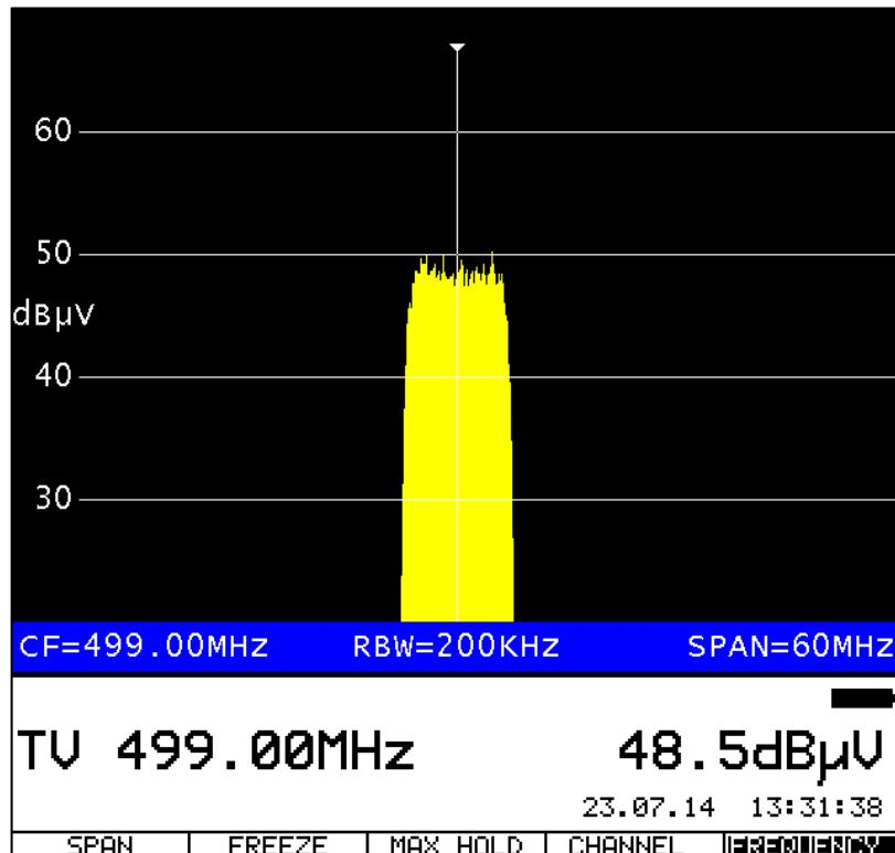
The measurement device shows a level of 48.5 dB $\mu$ V at the cursor position. However, if the device is tuned to the DVB-C channel (exit analyser) then this results in a level of 60.3 dB $\mu$ V as the following screenshot shows.
