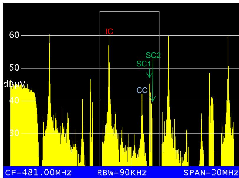
The peak value of the image carrier is measured per definition when measuring the level of an analogue TV channel. The KWS measurement devices use a measurement bandwidth of 200 KHz. Here the maximum must be determined within the period of a half image (peak detector).
