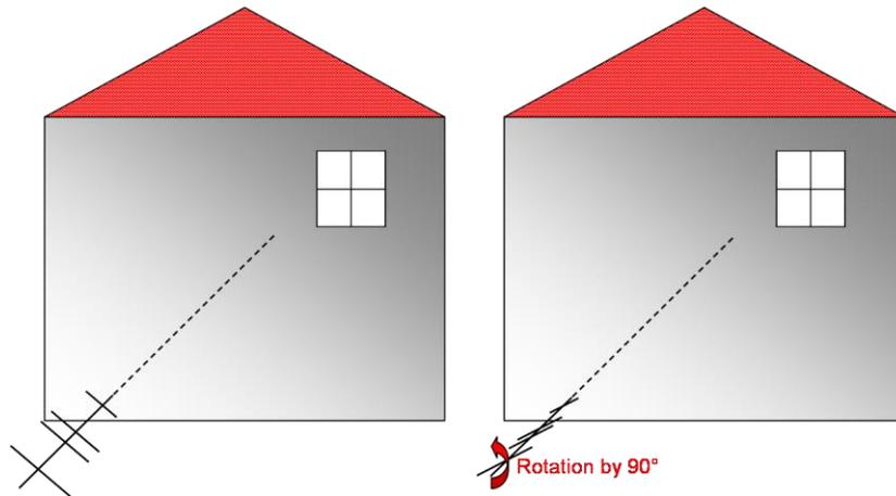
In order to locate maximum levels at the measurement location, the rod antenna must be aligned in all three spatial directions, as shown in the figure below.
